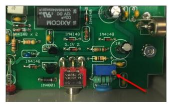
There is a short delay between the end of PTT assertion and when the transmit/receive switch returns to receive mode. The length of this delay is factory set but if necessary, the length of the delay can be adjusted. Remove the bottom cover of the Transmit/Receive switch and rotate the adjustment screw on the top of the trimpot clockwise to increase the delay time and counterclockwise to reduce it.
