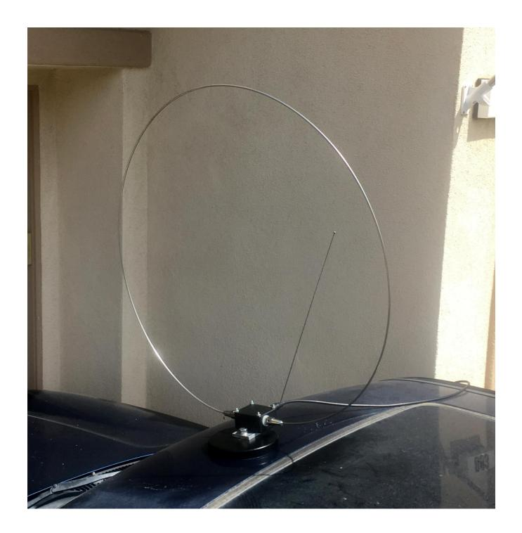
While being cautious about fingers, gently place the magnetic base at its desired location. The loop should be positioned such that the plane of the loop aligns with the vehicle.
