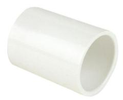
If a permanent extension to the lower 1" PVC pipe is necessary, a 1" to 1" PVC slip coupler can be used between the lower section of the antenna structure and the top of an appropriate length of 1" PVC pipe with both glued into the coupler. Use only the supplied 12 VDC linear power adapter or equivalent. Do not use a switching 12 VDC power adapter as it will inject noise into the received signals.
